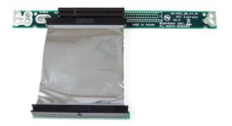
The PEX8RISERF x8 to x8 PCI Express Riser Card with flexible cable allows for installation of a x8/x4/x1 PCI Express (PCIe) card into a 1U rack mount or small form form factor chassis that would typically not allow cards to be mounted directly to the motherboard.
